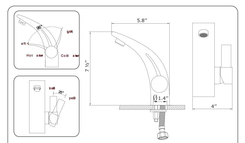
Make sure the installation holes are in the correct size. Install the lavatory and pop-up waste as shown in the drawing. Connect the main body and water supply pipe with water inlet pipe
