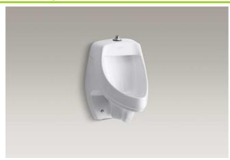
The siphon jet urinal shall be made of vitreous china with a 3/4" top spud. Urinal shall include inlet and outlet spuds and hangers. Urinal shall include antibacksplash wall. Urinal shall use 0.5 gpf (1.9 lpf) or 1.0 gpf (3.8 lpf). Urinal shall be WaterSense compliant when used with WaterSense flushometer. Urinal shall have a 14-1/2" (368 mm) extended rim.
