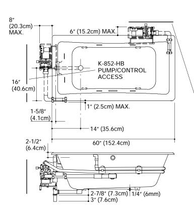
No change in measurements if connected with drain illustrated. (K-7169-AF or K-7169M-AF)
