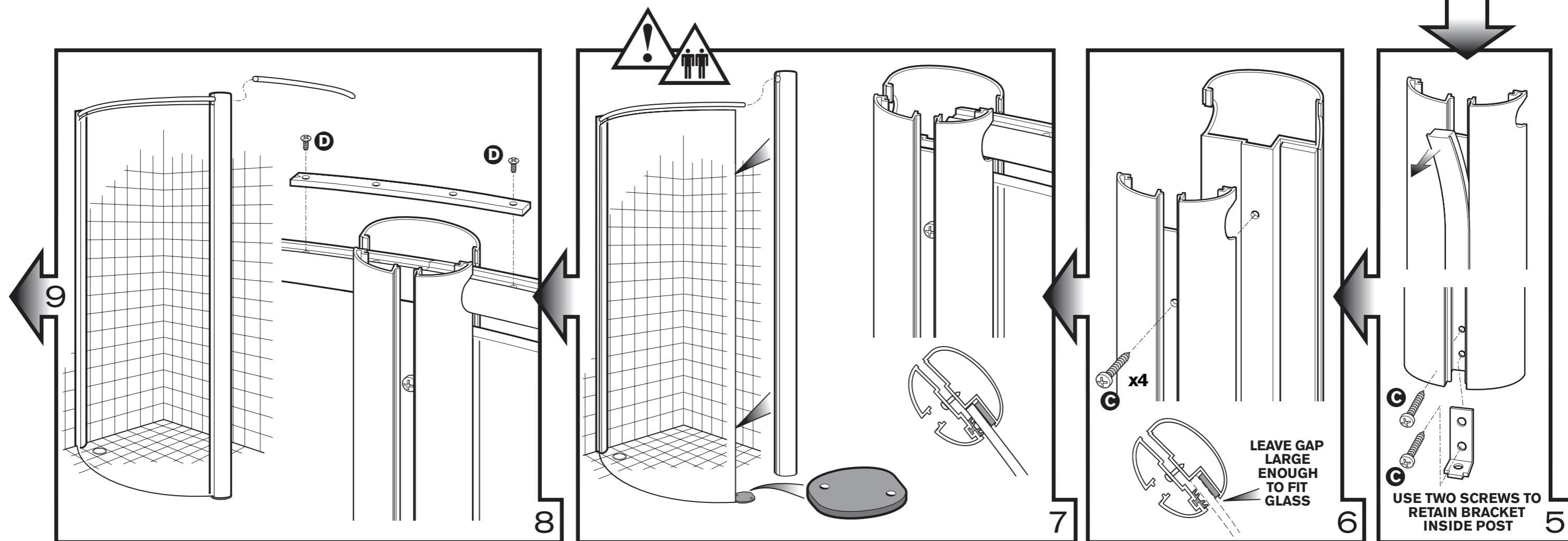
**ENSURE GLASS IS CORRECTLY LOCATED IN POST THEN FULLY TIGHTEN SCREWS**
