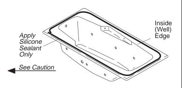
Carefully position the counter on the bath rim. Use braces, clamps, or weights to securely hold the counter in place until the sealant cures.
