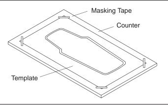
Determine the desired offset between the bath rim and the counter edge, and carefully cut the counter along the appropriate template cut line. Cut along the outside edge of the chosen template cut line.
