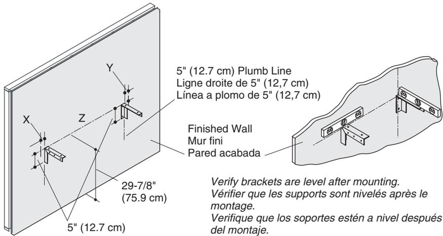
**NOTICE:** The mounting brackets are attached to the back of the unit. Prior to removing the mounting brackets, several dimensions must be recorded to ensure a successful installation. Use the table below to record these measurements.
