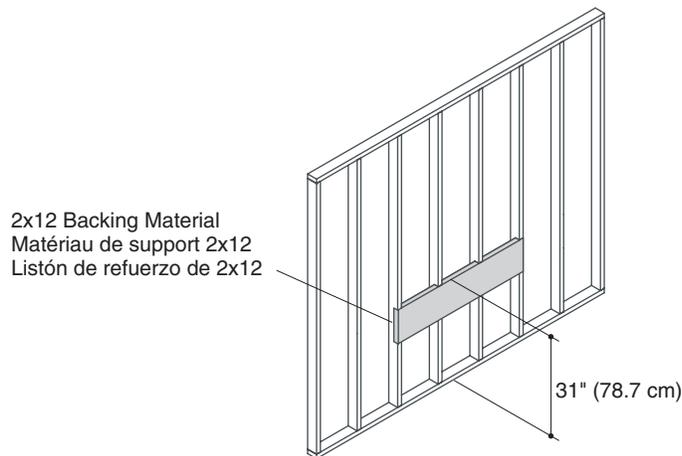
**NOTE:** The dimension provided is for a 34-1/2" (87.6 cm) vanity height. If an alternate height is desired, calculate the desired height of the backing material.
