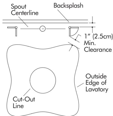
Cut out the opening by carefully following the pencil line.
