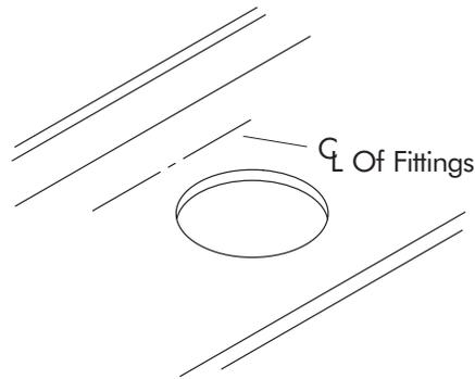
Clean the countertop, and carefully position the lavatory in the countertop opening so the “Kohler” logo is to the back. Line up the lavatory edges with the pencil line or masking tape border.
