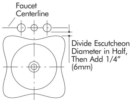
Carefully draw the calculated faucet centerline on the cut-out template. Choose the most suitable location based upon the following factors:
