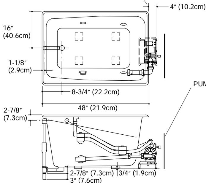
No change in measurements if connected with drain illustrated. (K-7163 or K-7163M)
