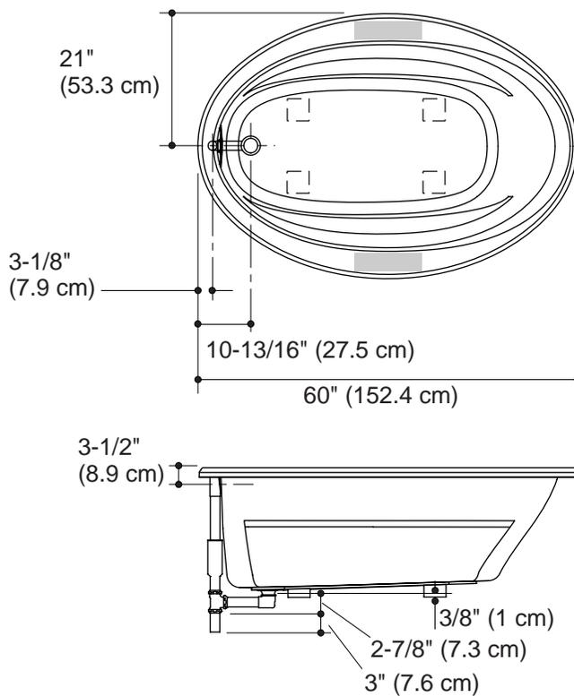
No change in measurements if connected with drain illustrated. (K-11677 or K-11677M)
