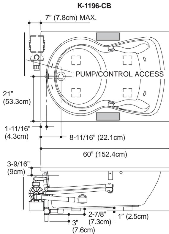
No change in measurements if connected with drain illustrated. (K-7161-AF or K-7161M-AF)
