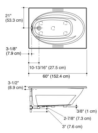
No change in measurements if connected with drain illustrated. (K-11677 or K-11677M)
