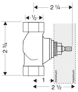
the surface of the finished wall must fall between the minimum and maximum lines.
