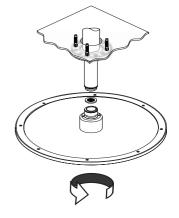
Secure the showerhead with the hollow set screws. (allen wrench = 2 mm)
