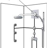
Three-function shower with Ecostat thermostatic mixer, 3/4" volume control, and Quattro diverter.
