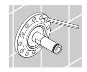
Drill the screw holes with a 6 mm drill bit suitable for the wall surface (1,2). Install the anchors (3). Seal the wall around the anchors with a waterproof bathroom sealant.
