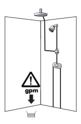
Two-feature installation with Ecostat thermostatic mixer and Trio diverter.
