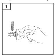
Locate water supply inlet and shut off water supply valve. Clean and dry surface area where new faucet will be mounted.
