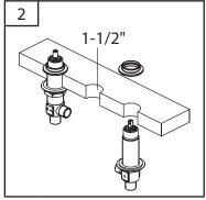
Drill three 1-1/2" holes into the tub deck no more than 15" on center. Place mounting nut, metal washer and rubber washer onto valve body. From underneath the tub, insert valve body through holes (Note: cold on the right side, hot on the left side). From above, thread flange onto valve stem. Tighten mounting nut, so that the flange sits flush to the surface of working area.
