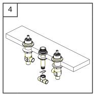
Insert tee onto shank until it is completly seated. Place clip through slot.
