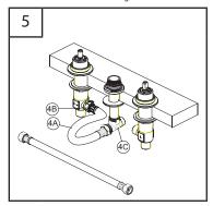
Connect the flexible water supply hose (4A) to the bottom of the valve body (4B) as shown. Align T-tube (4C) in a position which will allow maximum clearance to connect hoses. Carefully bend the hoses to fit the available space. Carefully thread the hose coupling to the side of the tee.
