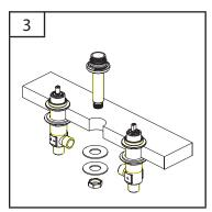
Place long shank through mounting hole in deck. Secure spout with rubber washer, metal washer and nut. Tighten nut securely with wrench.
