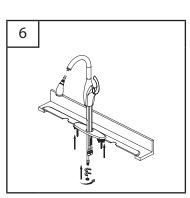
Hand tighten mounting nut onto bolt. Install rubber washer, metal washer and nut onto the mounting shank.
