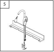
Install rubber washer, metal washer and nut onto the mounting shank.
