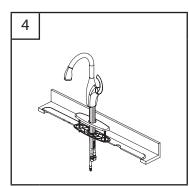
OPTIONAL ESCUTCHEON INSTALLATION Screw metal threaded rods upwards into cover plate and base plate on the sink. Insert faucet through mounting holes in sink.
