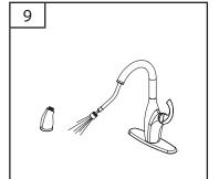
FAUCET OPERATION AND INSPECTION Turn on hot and cold water supplies. Pull the hose assembly out of the spout and remove the spray head. Be sure to hold the end of the hose down into the sink and turn faucet handle to the mixed position. Flush water lines for one minute. Check for leaks. Re-tighten if necessary, but do not overtighten. Reinstall the spray head.
