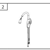
ATTACH SPOUT TO VALVE Feed hose assembly through spout and hub. Attach sprayer to end of hose to keep hose in place. Rotate spout assembly to ensure smooth operation.
