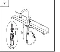
HOSE INSTALLATION Align block (1) onto hose. Install quick connect onto spray hose. Push quick connect firmly onto outlet hose tab. Install weights onto spray hose. Locate the weights 24" from the underside of the sink deck.
