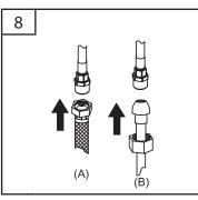
Connect water supply lines. (A) Use 1/2" IPS faucet supply lines or use coupling nuts (not supplied) with ball-nose risers (not included). Turn water supply or shut-off valve back on and check for leaks. If leaks occur, gently tighten the faucet connections.
