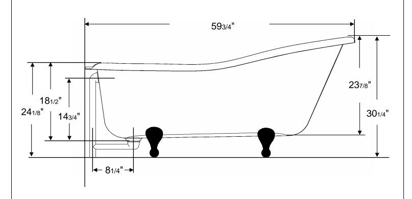
These dimensions are for reference only, and can vary +/- 1/4". If exact measurements are required, please use the actual tub to be installed.
