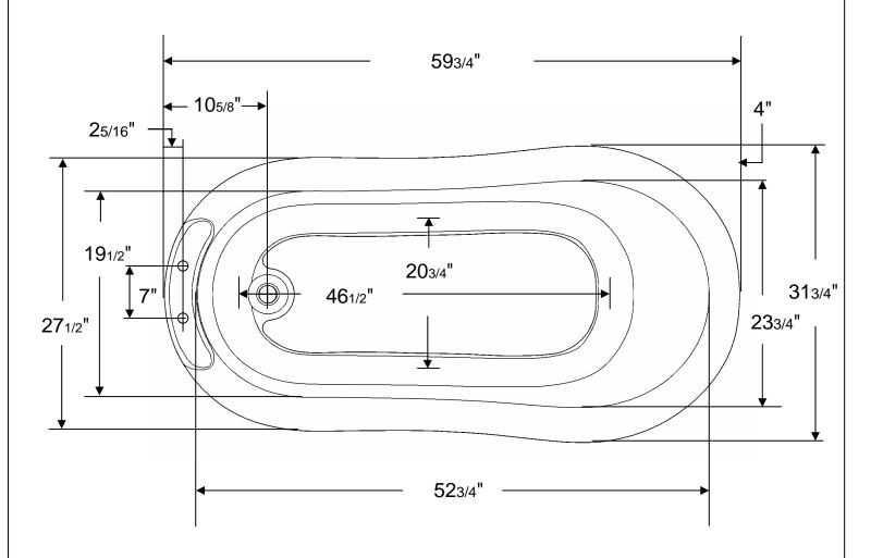
These dimensions are for reference only, and can vary +/- 1/4". If exact measurements are required, please use the actual tub to be installed.
