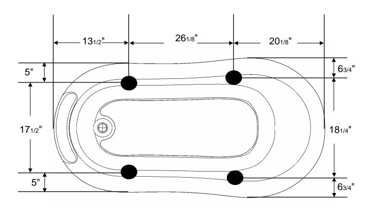
TheseDimensions are for reference only, and can vary +/- ¼". If exact measurements are required, please use the actual tub to be installed.
