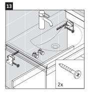
For wood stud wall, bolts should be screwed into wood backing.
