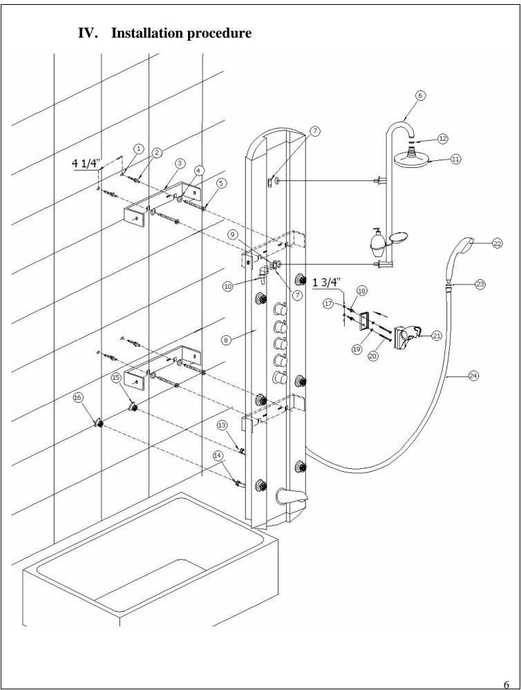
Refer to the technical diagram to choose the proper location for your shower column. You can adjust the column's vertical position based on the person's height. (Measurements given in the technical diagram are based on the average human height -68"-70").
