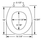
Ring thickness is 3/8" Ring thickness including the bumper is 5/8" Height of the seat with cover is 1-1/2" Seats shall be No. 70 as manufactured by Church Seats. Seats shall be standard weight and injection molded of solid plastic. Seats shall be closed front with cover for round bowl and feature molded-in bumpers. Color-matched hinges with non-corrosive top-tightening bolts and wing nuts. Color to be\_\_\_\_\_\_\_. (specify white or fixture manufacturer's color)
