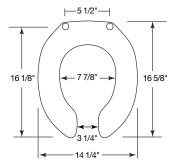
Ring thickness is 13/16" Ring thickness including the bumper is 1" Height of Seat is 2-1/4"
