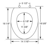
Ring thickness is 3/8" Ring thickness including the bumper is 5/8" Height of the seat with cover is 1-1/2" Seats shall be No. 170 as manufactured by Church Seats. Seats shall be standard weight and injection molded of solid plastic. Seats shall be closed front with cover for elongated bowl and feature molded-in bumpers. Color-matched hinges with non-corrosive top-tightening bolts and wing nuts. Color to be \_\_\_\_\_\_. (specify white or fixture manufacturer's color)
