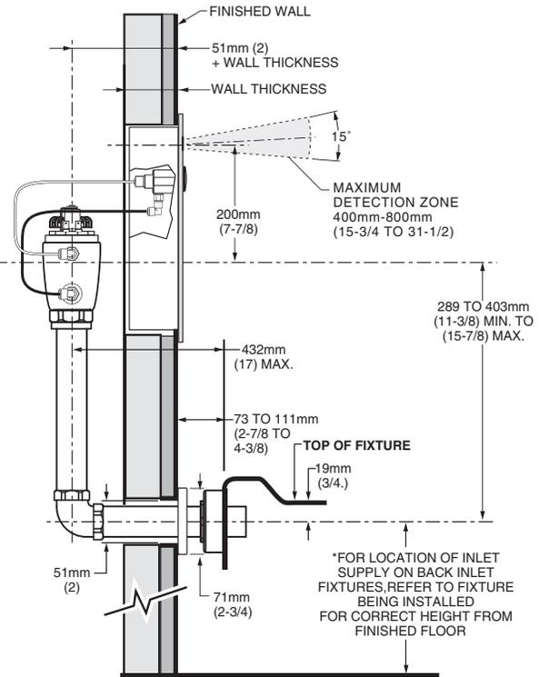
\*Note: The Critical Line (-C-L-) on Vacuum Breaker must typically be 6" (152mm) min. above fixture. Consult Codes for details.
