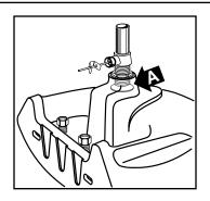
Return the fitted lavatory and pedestal to the installed position. Connect trap to drain assembly hand tight to check alignment. It may be necessary to cut off part of the tailpiece (area "B") and/or part of the drain elbow of the trap (area "C").
