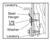
IMPORTANT: Final assembly of nut and washer or lag bolt method shown for reference only. (See steps 8 and 9).
