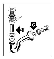
Secure lavatory to wall as shown in **5** or **5a.** Install washers and hand tighten nuts or lag bolts.
