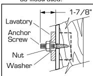
LAG BOLT INSTALLATION Use lag bolts to secure lavatory as illustrated.
