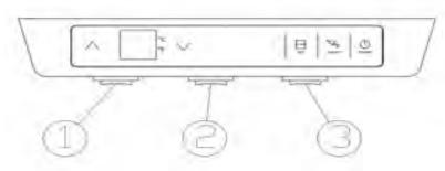
Light switches are under the control panel to control the lights turn on/off:
