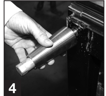
4 Thread leg into cabinet bottom frame rail.
