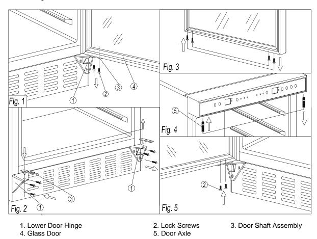
**NOTE:** All parts removed must be saved to allow the door swing to be reversed.
