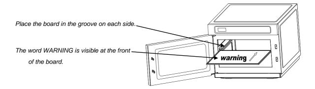
3. Be sure the ceramic board has been pushed all the way to the back of the cavity. If you do not install it correctly, the door cannot be closed.
