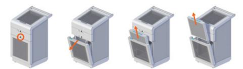
Marking on the Defend 1050 unit corresponding with the required filter.
