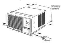
2 Slide the unit from the cabinet by gripping the base pan handle and pulling forward while bracing the cabinet.
