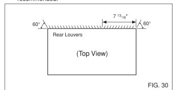
If the wall sleeve already has a rear grille, skip to step 4. If the wall sleeve does not have a rear grille or louvered panel, install the plastic grille from the kit. Cut the plastic grille to 26-1/2" wide and 15-1/2" high or to the sleeve dimensions. Place the plastic grille to the inside of the wall sleeve at the rear flange.
