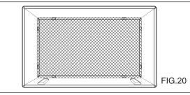
2 Fasten the 4 washer screws to secure the grille to the wall sleeve. If you need plastic nuts to mount plastic grille to the inside of the wall sleeve, there are plastic nuts in the installation kit. The nuts are installed from the inside of the sleeve and are pressing into the square holes of the rear flanges.Fasten the bracket to the upside of the wall sleeve using the washer screw. The bracket prevents the unit from leaving the sleeve.
