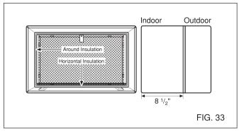
If the depth of your existing sleeve is less than or equal 5 to 18", skip to step 7. Otherwise, cut the baffles and the support blocks according to Length "A" in the table below.
