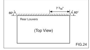
2 If the wall sleeve already has a rear grille, skip to step 4. If the wall sleeve does not have a rear grille or louvered panel, install the plastic grille from the kit. Cut the plastic grille to 25-1/2" wide and 15-1/4" high. Place the plastic grille to the inside of the wall sleeve at the rear flange.
