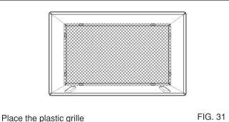
Fasten the 4 washer screws to secure the grille to the 3 wall sleeve. If you need plastic nuts to mount plastic grille to the inside of the wall sleeve, there are plastic nuts in the installation kit. The nuts are installed from the inside of the sleeve and are pressed into the square holes of the rear flanges. Fasten the bracket to the upside of the wall sleeve using the washer screw. The bracket prevents the unit from leaving the sleeve.
