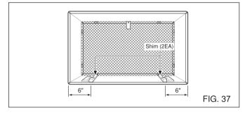
8 Install the new unit into the wall sleeve
