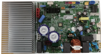
LMU183HV (18 kBtu/h) and LMU243HV (24 kBtu/h) Main PCB
