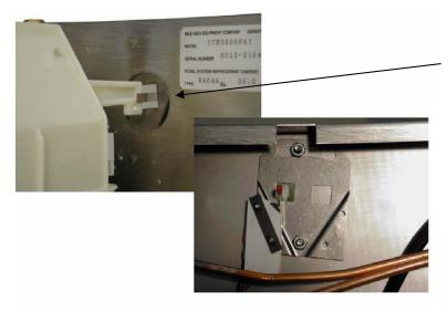
Water splash curtain actuator tab positioned behind bin switch
