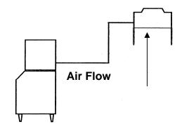
DO NOT Install any part of the refrigerant lines below the quick connect fittings at rear of machine.
