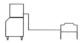
**DO NOT** Install the condenser lower than 6' (1.83 meters) below the quick connect fittings at rear of machine.
