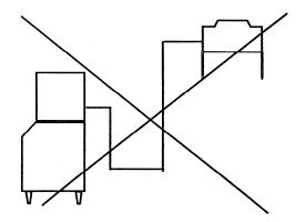
When installing condenser below the ice machine
