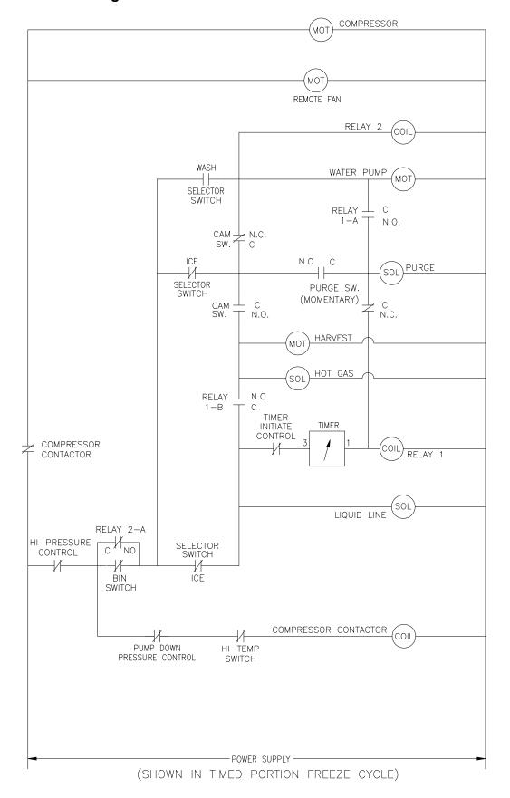
ICE0606 Air3 and Water3, ICE0605 Air3 and Water3 Wiring Diagram ICE0806 Air3 and Water3, ICE0805 Air3 and Water3 Wiring Diagram ICE1006 Air3 and Water3, ICE1005 Air3 and Water3 Wiring Diagram
