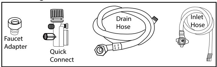
Your dishwasher comes equipped with a Faucet Adapter, Quick Connect, Drain Hose, and Inlet Hose. The Faucet Adapter must be installed on the faucet before you can connect the dishwasher. This adapter comes packaged inside your dishwasher.
