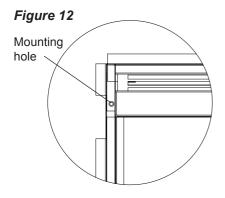
in each corner of the fireplace chassis, into wall studs (Figure 12).
