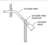
Thread swivel connection on to your present shower arm. Be sure all gaskets are in place. Attach shower head onto end of diverter in-line with shower arm. Attach hose to fitting 90° from center-line of shower head. Tighten all fittings and your shower is ready to use.
