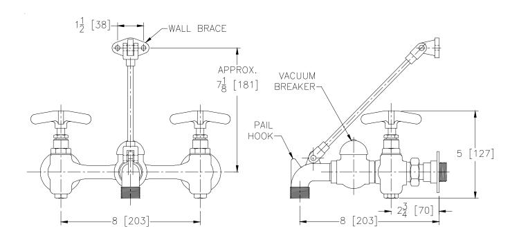
**Z1996-SF Service Sink Faucet -** Chrome plated service faucet, complete with vacuum breaker, integral stops, adjustable wall brace, pail hook, four-arm hot and cold handles and 3/4 [19] hose thread on spout. Water inlets are for 1/2 [13] pipe and are eccentric on an 8 [203] centerline.
