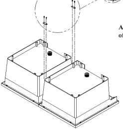
Insert the metal connector brackets into the leg slots as shown. Tap gently with a hammer if the fit is tight. Insert the four legs in the four remaining leg slots.
