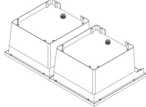
Attach the plastic connector to the four towel bar lugs on the underside of the sinks using the four screws provided.
