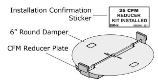
**2.** Position CFM reducer so that reducer clips hang over blower collar.
