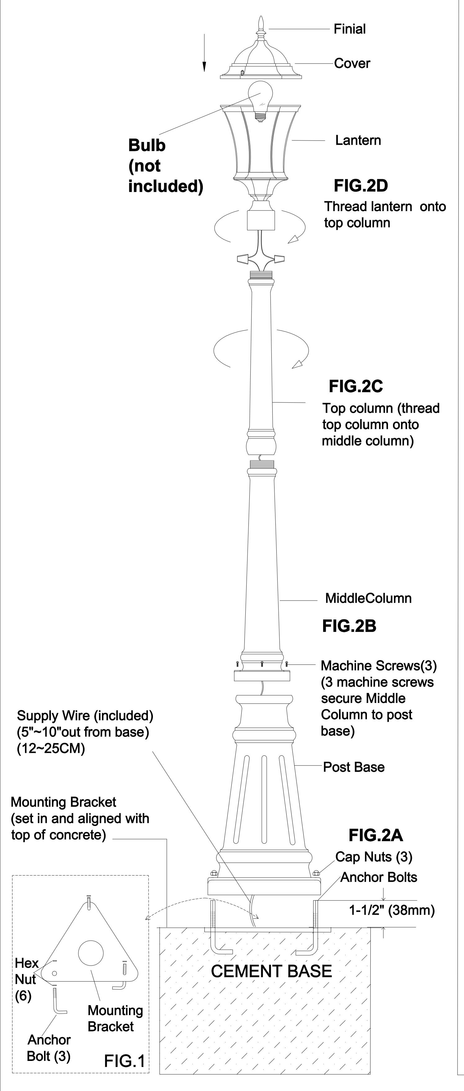
Before starting the installation, disconnect the Power by Turning Off the Circuit Breaker. Turning the Power Off using the Light Switch is not sufficient to prevent electrical shock. All electrical connections and installation must be in accordance with local codes, ordinances and/or National Electric Code and Must Be Done by an Electrician Only.
