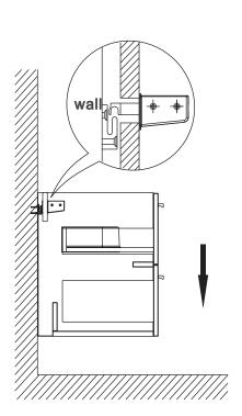
4 Adjust the mounting attachment as required
