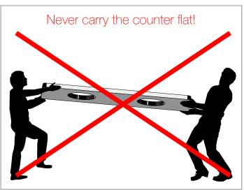
1 Lift the counter (using two people for counters 50" or larger) from the front side, leaving the back side on the bottom of the box. Bring to a vertical position.
