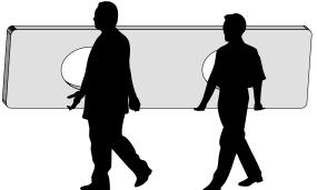
3 When installing the counter on the cabinet it is important to lift carefully, ensuring that the counter does not strike the cabinet, while still maintaining the vertical positioning. Counters can be heavy, so don't attempt this if you are not capable of handling the weight. While lifting the counter up and over the cabinet, gently place the back side of the counter close to the back of the top of the cabinet while standing to either side of the cabinet.
