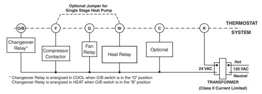
Figure 2. Typical wiring diagram for single transformer single stage systems
