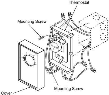
Note: Breaks both sides of line in "OFF" position
