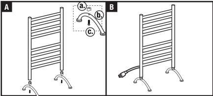
After installation is complete, connect the 5 foot electric power cord and turn on the Power Switch. The unit will begin to heat. If the unit will not be used for an extended time, simply turn the unit off using the power switch.
