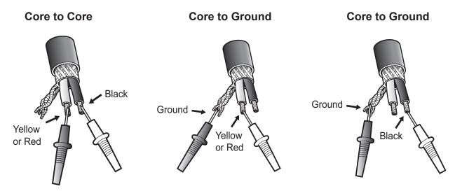
The ground wire may differ from the images above. The ground wire may be represented as a additional wire with a stripe. The testing procedure is still performed the same way.
