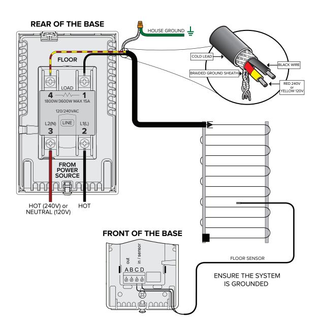
Figure 1. Wiring Diagram for 120V or 240V WarmlyYours TempZone™ Floor Heating Cable Installation
