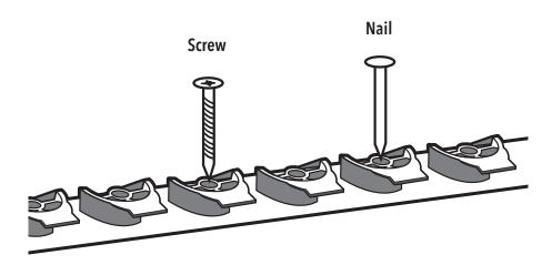
Figure 6. Securing the Cable Fixing Strips
