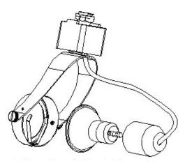
Push lamp into socket, then twist. Seat lamp under the "V" spring
