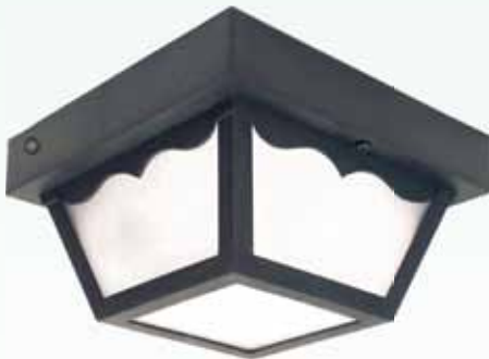
V6261-5 Black Polycarbonate Frosted Acrylic 8¼"W x 4¾"H 1x13W G24q-1 Base 120V NPF Electronic Ballast Photocell Included
