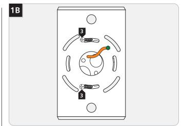
Attach the mounting plate to the electrical box using the two provided #8-32 screws .
