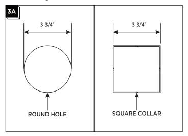
Mark an appropriate sized diameter circle or square on drywall. Cut out the marked section. **Note:** The drywall may be cut by running a 1/8" RotoZip around the outside of the collar or inside round hole.
