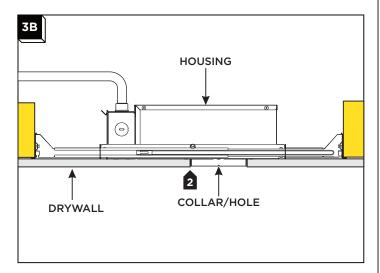
2 Align the cut out section of drywall with the collar/hole and install drywall.
