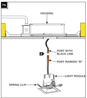
Connect the jumper cable to the housing wire making sure the port marked "B" is paired with the port with a black line.
