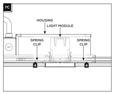
4 Release the spring clips to secure in place
