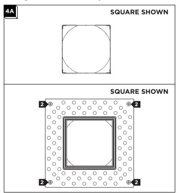
Install the provided 6x20 self-drilling screws through the plaster plate and housing at the marked locations. Do not place screws at any of the other mud holes on the plate.
