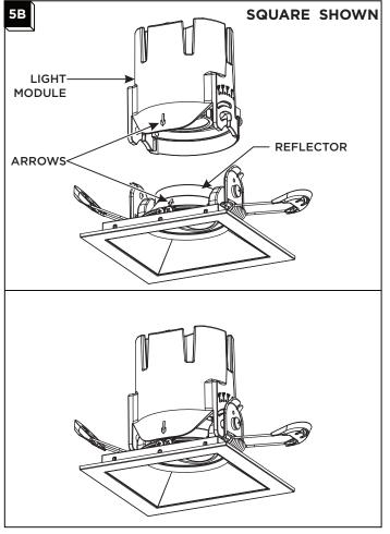
Carefully snap light module and reflector together. Alignment arrows are provided on the adjustable versions. Directional alignment is not required for fixed Versions.
