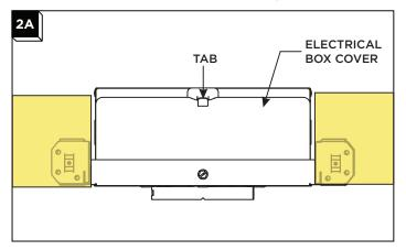
1 Push the tab on the housing electrical box up and remove the electrical box cover.
