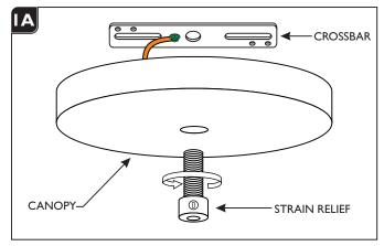
Remove the crossbar from the canopy by completely unscrewing the strain relief.
