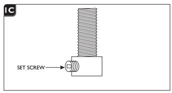
**13** Loosen (**Do Not Remove**) the set screw on the strain relief.
