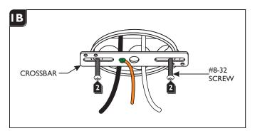
Mount the crossbar assembly to the electrical box with the two provided #8-32 screws.
