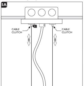
Adjust the aircraft cables until the fixture is level; feed the cable into the cable clutch to raise the fixture and push in on the cable clutch nipple to release the cable and lower the fixture.
